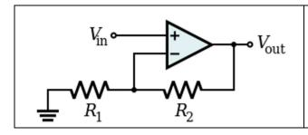
For existing monitoring systems still employing the 1.0V=1.0mW scale, the following op-amp circuit can be used to scale the new Vmon output. Resistor values of R1=1.0k $\Omega$  and R2=9.0k $\Omega$  will multiply the Vmon reference voltage by 10x and make the signal compatible with old scale monitoring systems.
