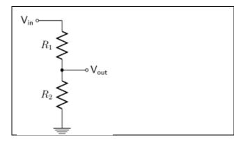
For new monitoring systems that incorporate the new 0.1V=1.0mW scale, a simple resistive voltage divider circuit can be implemented for older equipment still using the previous 1.0V=1.0mW scale. Resistor values of R1=10k $\Omega$  and R2=1.1k $\Omega$  will provide the necessary voltage scaling of 1/10. Any voltage divider circuit that reduces the input voltage by a factor of 10x can be used.
